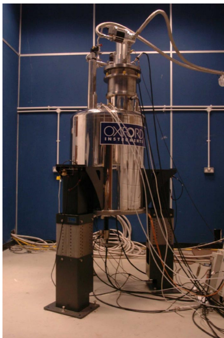
FIG. 1. (Color online) 400 MHz NMR cryostat actively cooled by a Pulse Tube Refrigerator.
